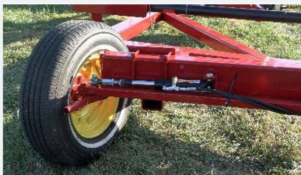
Hydraulic steering cylinder enables easy maneuvering.
