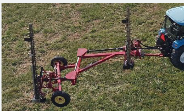
Hydraulic steering cylinder enables easy maneuvering.
